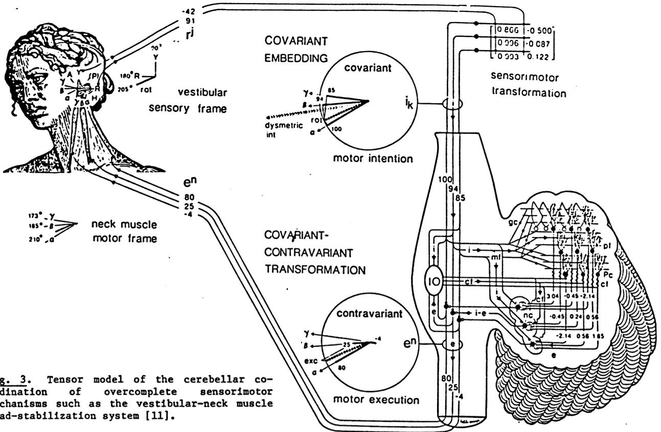
Fig. 3. Tensor model of the cerebellar coordination of overcomplete sensorimotor mechanisms such as the vestibular-neck muscle head-stabilization system [11].
